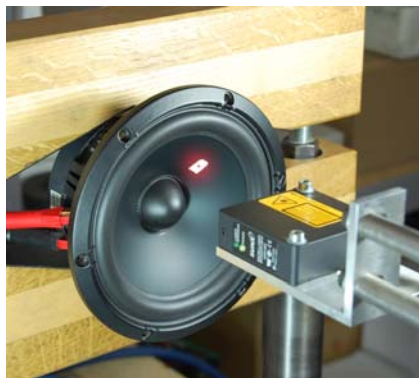
Excursion measurements with a high precision laser sensor
